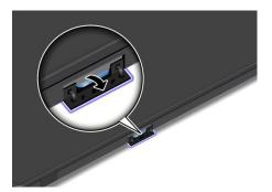
4. If a SIM card is preinstalled in the slot, push the SIM card inward a little, the SIM card pops out. Gently slide the SIM card out of the slot.
